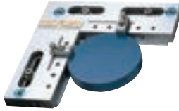
Large work-piece - Clamp on
