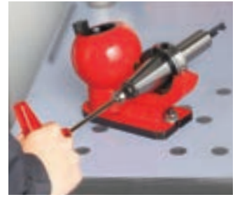
Clamping DETa-1 Collet( DTB )
