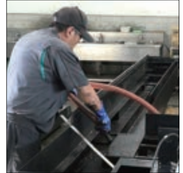
Periodic cleaning of the coolant tank
