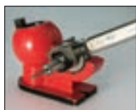
Adjustable torque wrench The nut-tightening torque can be adjusted more properly. P. 31
