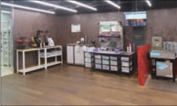
Centralized management of cutting tools and holders in tool room
